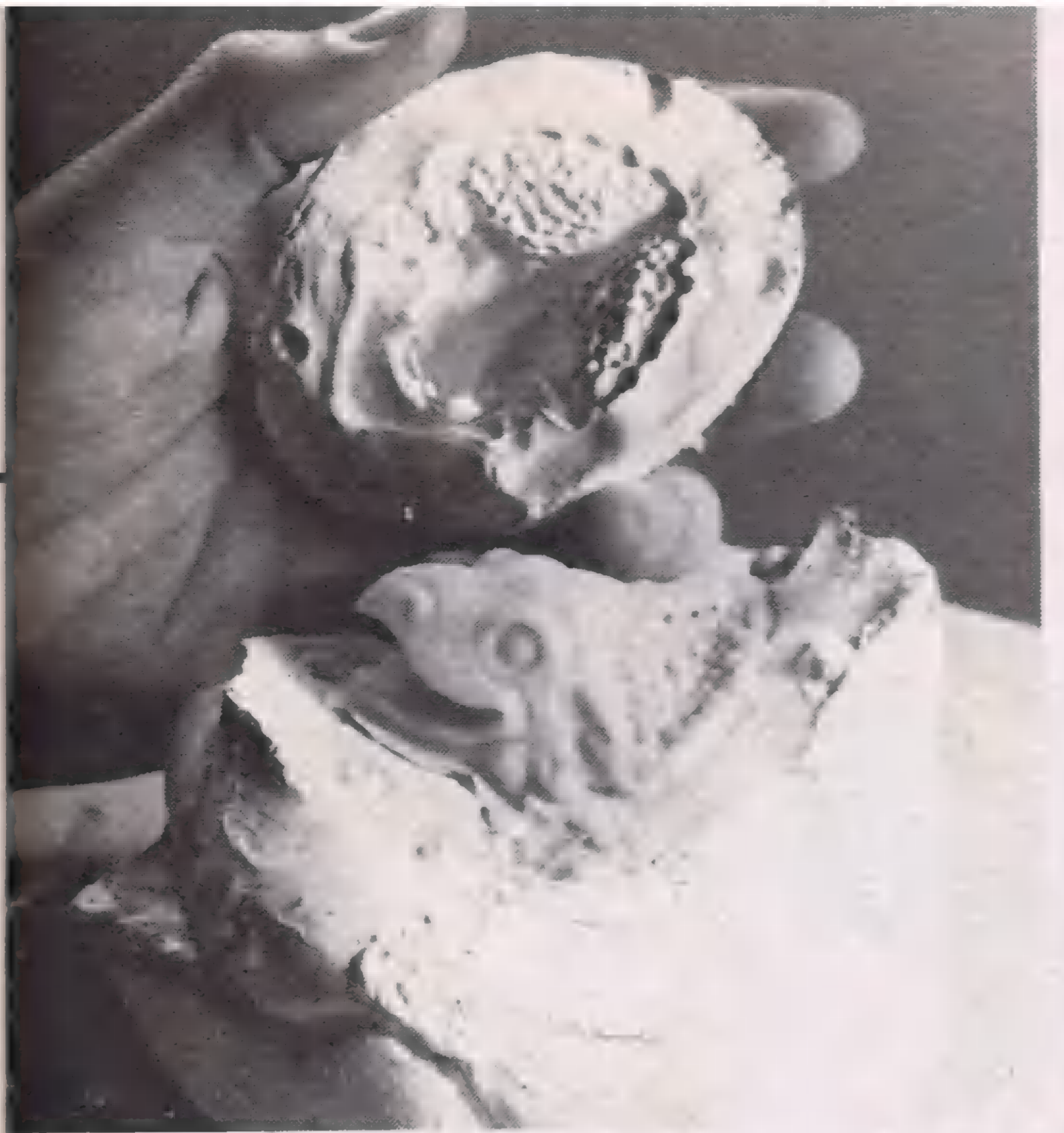
The hollow shell-casting was made by pouring latex rubber into the closed mold, letting it sit there for 60 minutes to allow a skin to build up on the mold interior. The extra rubber is poured out before final curing and vulcanizing the rubber for several hours in a 225 degree oven.
